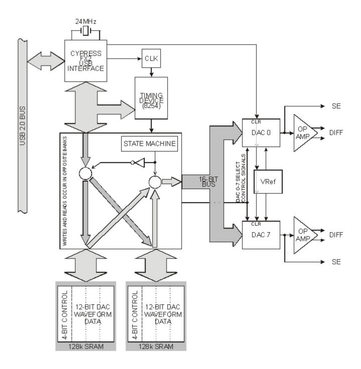
Figure 1-1: Block Diagram
