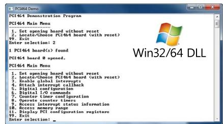
For Windows 8 / 7 / Vista / XP • Supports Acromag XMC, PMC, PCI, CompactPCI cards ◆ Includes DLLs
