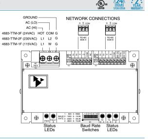
For N2 or BACnet MS/TP bus ◆ Drives up to 32 RS-485 devices ◆ Isolates and boosts signal up to 4000 ft.
