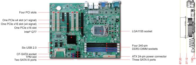
RUBY-D714VG2AR is based on Intel Q77 chipset and desktop processor sku like Core™ i7 and i5. Built with flexible PCI express expansion and bifurcation feature, it can support two I/O interface cards and can also suitable for Medical, Industrial Automation, and Digital Signage applications.
