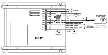
\* P1-8 & P1-12 user input may be programmed for a number of functions. Including (jog, inhibit, etc.)
