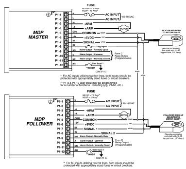
\*\* P1-8 & P1-12 user input may be programmed for a number of functions. Including (jog, inhibit, etc.)
