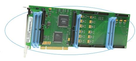
The APC8620A carrier card holds up to five plug-in I/O modules for extremely high channel density.
