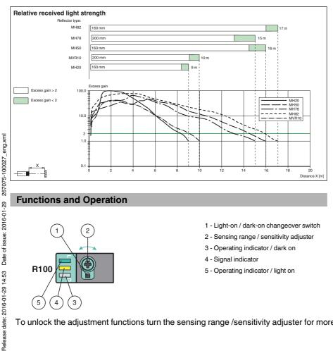
To unlock the adjustment functions turn the sensing range /sensitivity adjuster for more than 180 degrees.
