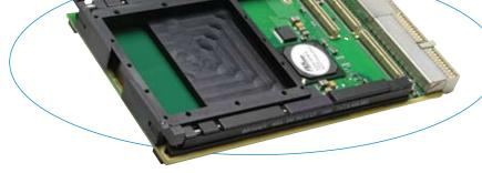
This conduction-cooled carrier card interfaces a PMC module to a CompactPCI computer system
