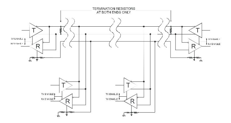
Figure A-1: Typical RS485 Two-Wire Multidrop Network
