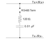
Figure 3-2: Simplified Termination Schematic
