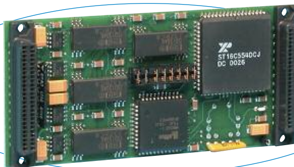
Large 64-byte FIFO buffers reduce the processing burden on the CPU to increase the overall system performance.
