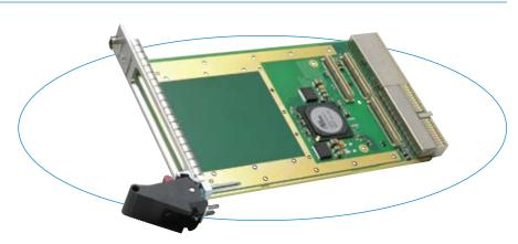
This carrier card interfaces a PMC module to a CompactPCI computer system.
