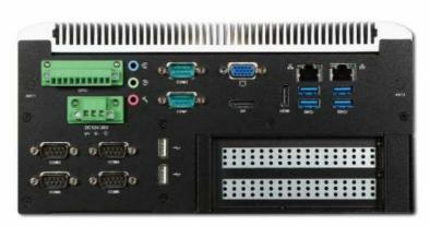
The WEBS-35C3 builds on Intel® desktop Q170 chipset and takes advantages of Intel® Core™ i3/i5/i7 desktop processor technologies that can support dual DDR4 memory. Support two Gigabit Ethernet ports, different add-on card expansion options, one M.2 socket and one Mini-PCle socket. The WEBS-35C3 is an ideal platform with rich I/O and high resolution for POS, kiosk, digital signage, and surveillance security monitoring applications.
