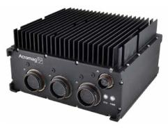
Air-cooled configuration (800 LFPM required) with finned heatsink provides consistent heat extraction from the double-wide ARCX System without the need for a cold plate.
