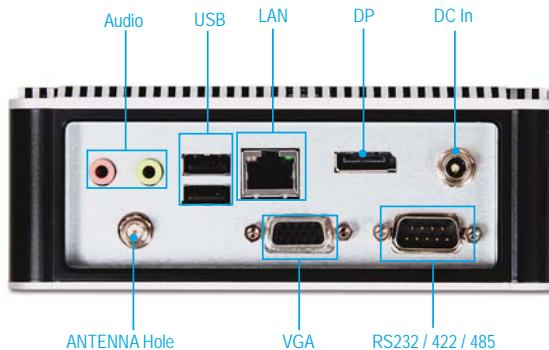
WEBS-2170 adopts latest Intel® AtomTM D2550/CPU and NM10 chipset which is for the low power compact size system. The new architecture integrates the 3D graphics engine and memory controller. It's suitable for Kiosk, DS and Networking applications.
