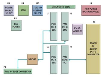
One PMC mezzanine module slot ◆ Non-Intelligent carrier card ◆ PCIe x4 interface
