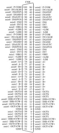
\* Axis0 - Axis3 of this manual corresponds to Axis No.1 - Axis No.4 in API-SMC(WDM).
