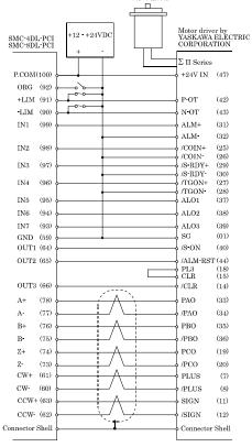
\* Please connect the Shield Line of cable with the Connector Shell.
