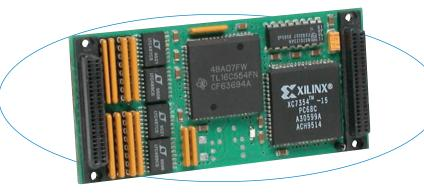
Large, 128-byte FIFO buffers reduce the processing burden on the CPU to increase the overall system performance.
