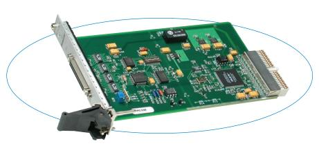
Advanced memory management techniques allow the AcPC330 to operate with minimal interruption of the A/D converter.
